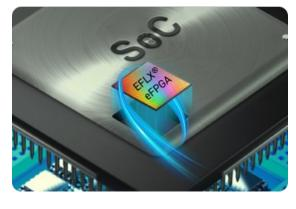
eFPGA may be used also for implementing the entire hybrid mechanism in a resource efficient manner. The eFPGA can be first programmed to implement a PQC KEM and to compute the PQC shared secret, next to implement ECC and to compute the ECC shared secret, and finally programmed to implement the key derivation function that computes the final shared secret from the PQC and ECC shared secrets.
